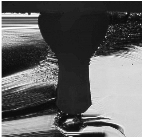
Figure 4-4: Resulting nozzle of a combination of isotropic and directional etching
