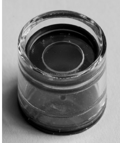
Figure 3-10: Filter module inside the glass tube package
