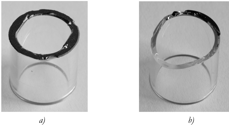
Figure 3-6: Glass tube package after burst pressure test. (inner and outer diameter are 13mm and 16mm )
